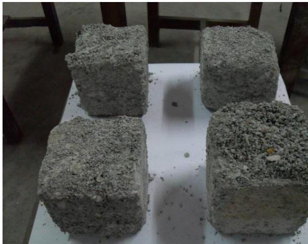
Plate no. 8: OPC Concrete specimens after 90 cycles of freezing and thawing in SW
