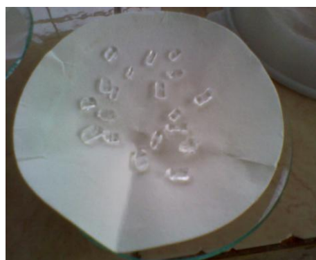
Fig. 1: Seed crystals of 85 ml NaCl doped KDP crystal.
