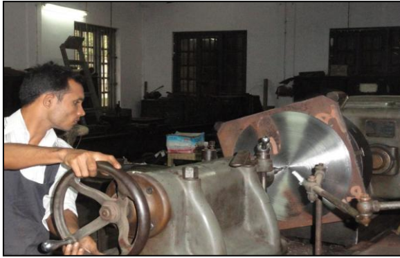
Fig. 5: Turbine runner disk is faced by lath machine
