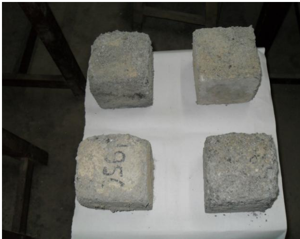
Plate no. 4: OPC Concrete specimens after 30 cycles of freezing and thawing in SW
