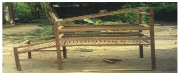
Fig. 2. Completed solar cabinet dryer – 2 m 2 models [6].
