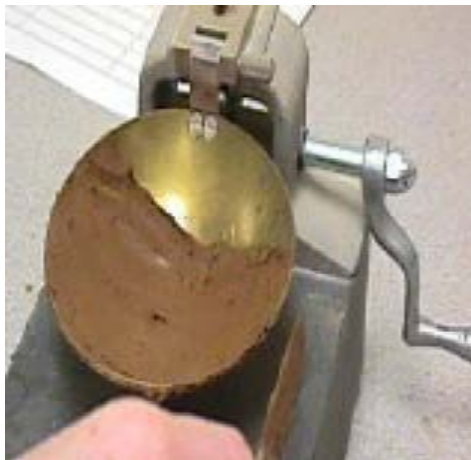
Fig: 1: Casagrande method of determining liquid limit
