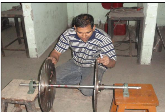
Fig. 7: Runner end pieces are attached on shaft
