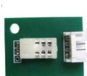
Figure.9: Humidity sensor (HSM 20G).
