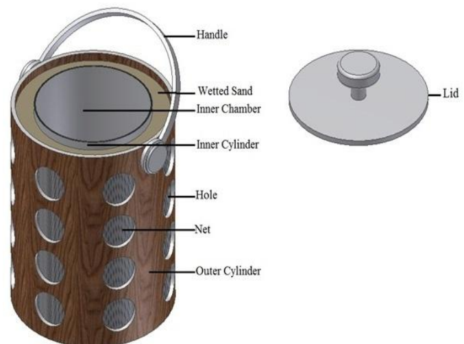
Fig.2: Construction of solar powered refrigerator
