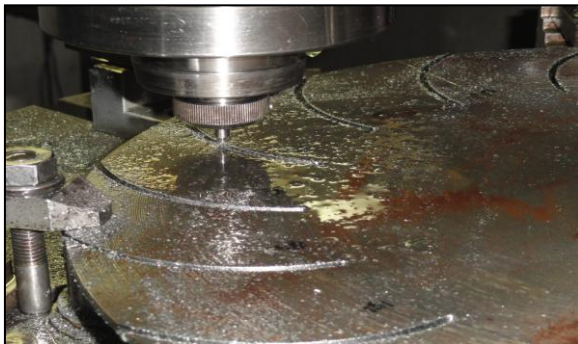
Fig. 6: Cutting of blade profile on runner disk by Jig boring machine
