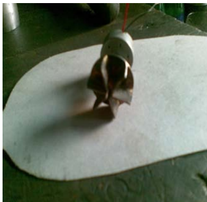
Fig.9: DC motor coupled with impeller
