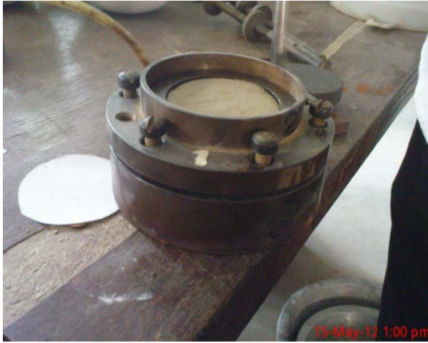
Fig.1: Soil specimen in consolidation cell
