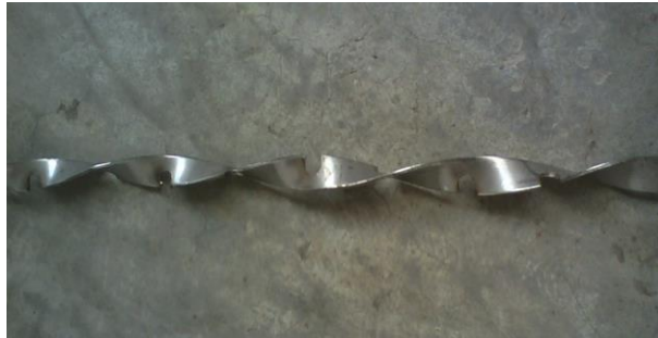
Fig. 2(a): Photograph of U-cut twisted tape
