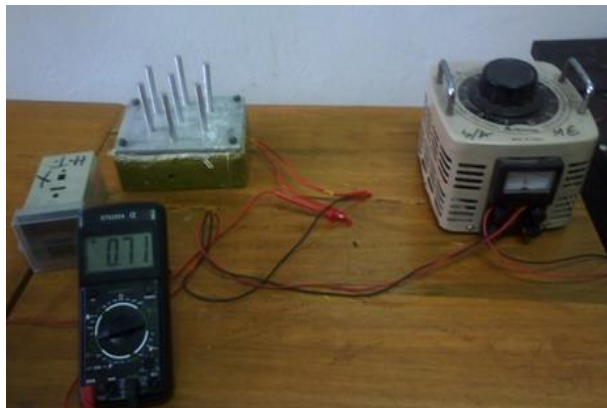
Fig. 2: Assemble of fin for free convection.
