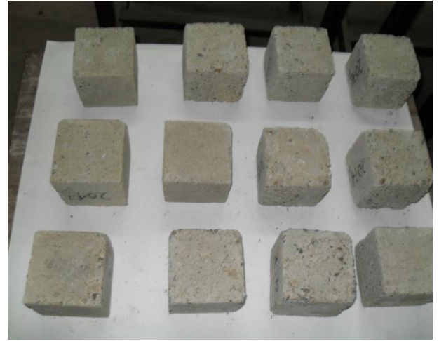
Plate no. 3: FA Concrete specimens after 30 cycles of freezing and thawing in PW
