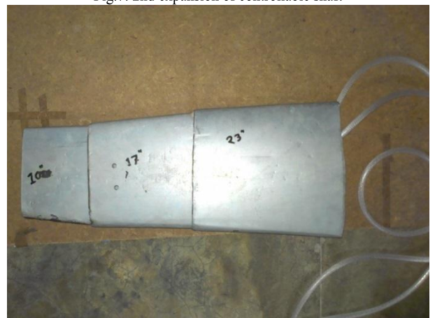
Fig.8: 2nd expansion of controllable wing
