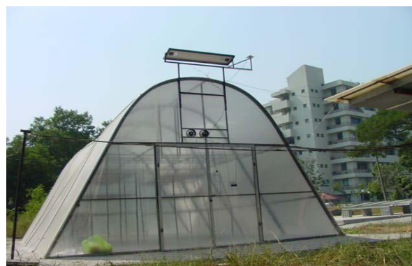
Fig. 8. Pictorial view of the greenhouse solar dryer solar dryer with polycarbonate sheet [7].
