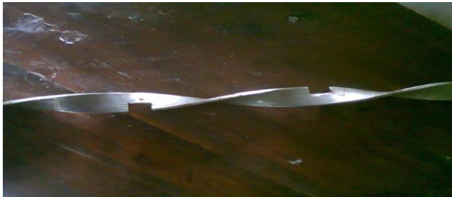
Fig 2.3: Twisted tape strip with 9 rectangular cuts (Insert 1)
