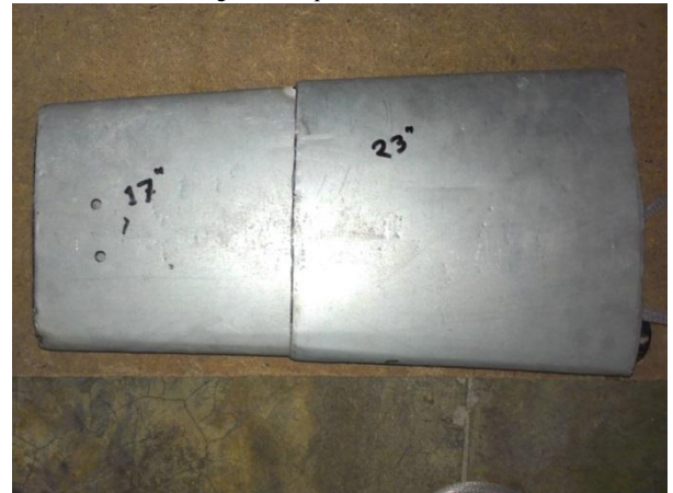
Fig.6: 1st expansion of controllable wing
