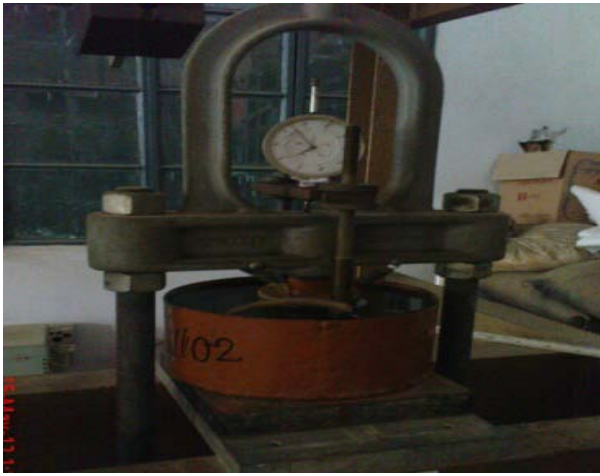
Fig.2: A consolidation cell during experiment
