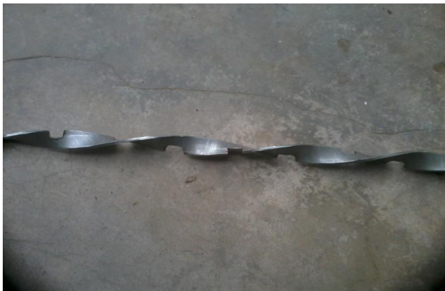
Fig 2.4: Twisted tape strip with 18 rectangular cuts (insert 2)
