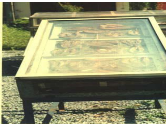
Fig. 4. Fully assembled box dryer [10].
