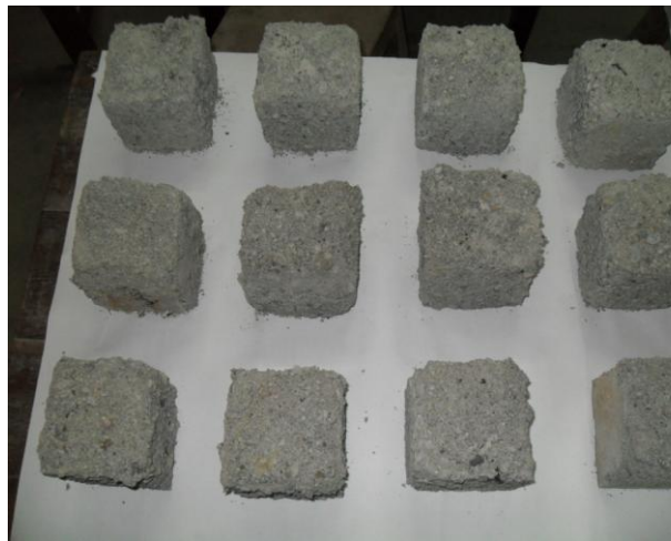
Plate no. 9: OPC Concrete specimens after 90 cycles of freezing and thawing in SW
