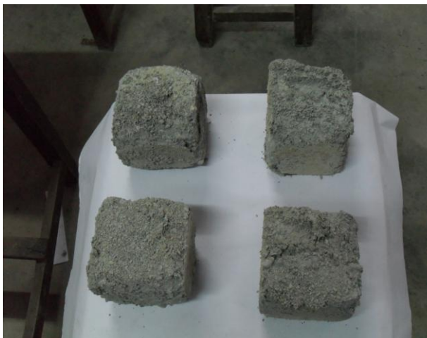
Plate no. 6: OPC Concrete specimens after 90 cycles of freezing and thawing in PW
