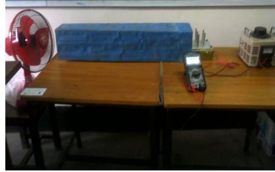
Fig. 3: Assemble of fin for force convection.
