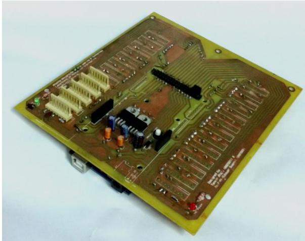
Fig. 4: Arduino board with shield for connecting transducer cards.
