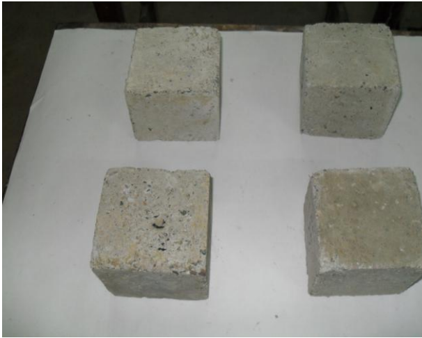
Plate no. 2: OPC Concrete specimens after 30 cycles of freezing and thawing in PW
