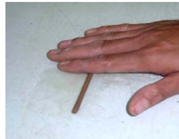
Fig: 2: plastic limit determination
