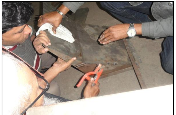
Fig. 9: end pieces of nozzle are jointed together and spot welded.
