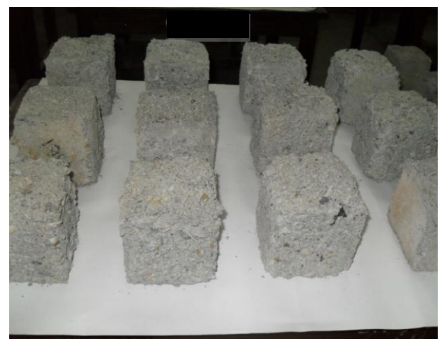
Plate no. 7: FA Concrete specimens after 90 cycles of freezing and thawing in PW
