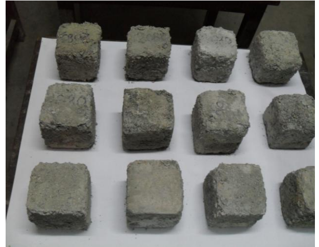
Plate no. 5: FA Concrete specimens after 30 cycles of freezing and thawing in SW
